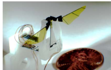
Fig. 2. Three DOF (degree of freedom) 3cm flapping wing MAV
